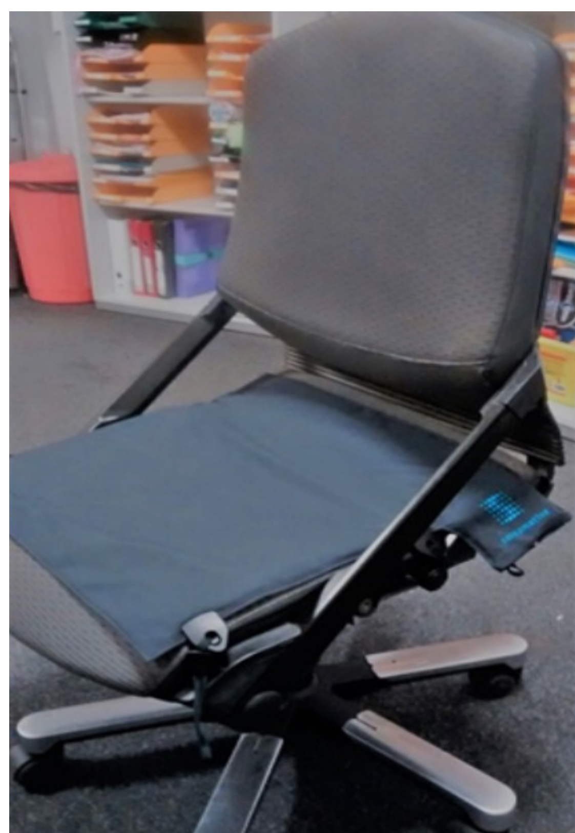
Figure 2. Office desk chair with sensomative pressure mat.
