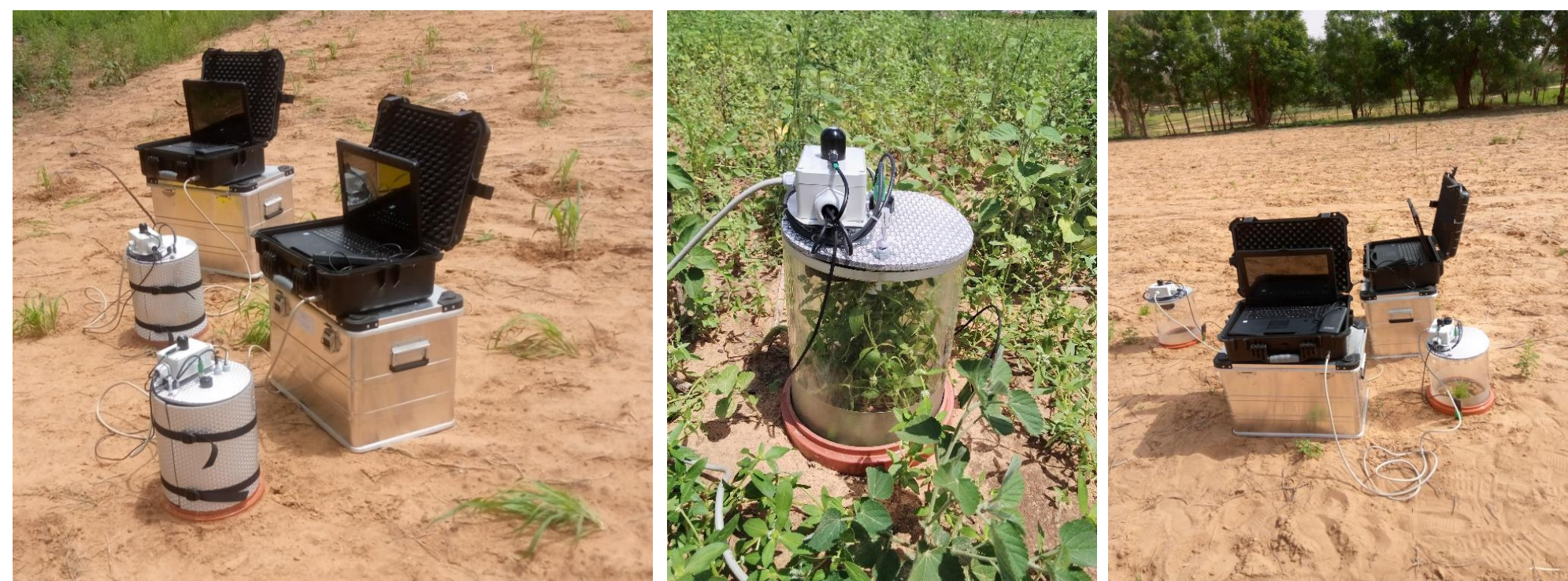
Fig. 2: SEMACH-FG closed chamber systems
